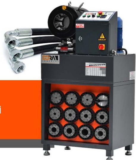
HİDROLİK HORTUM SIKMA ve BORU AĞZI BÜZME PRESİ HYDRAULIC HOSE CLAMPING AND PIPE BRACKET PRESS
